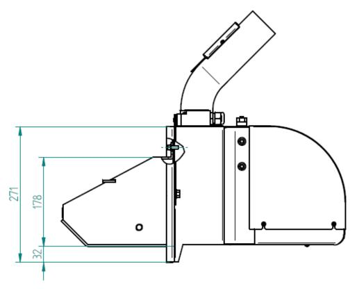
**Figure 4.2.** Overall and characteristic dimensions of the main unit – *side view*;
