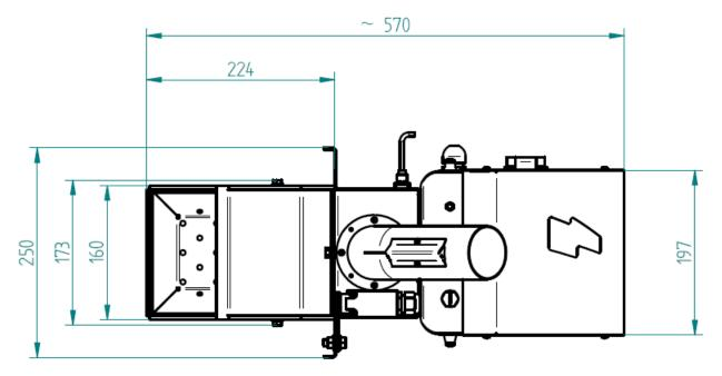
**Figure 4.3.** Overall and characteristic dimensions of the main unit – *top view*;
