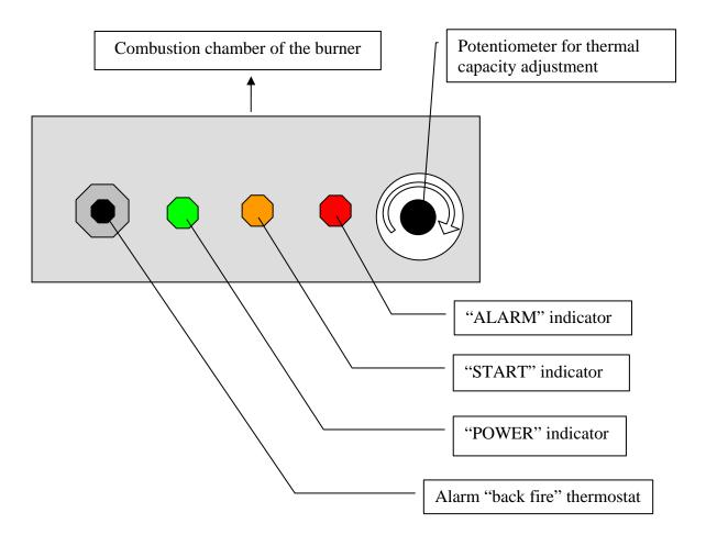
**Figure 5.1.** Interface board, equipped with indicator lamps, control and safety elements of automatic pellet burner "ERATO GP20+".
