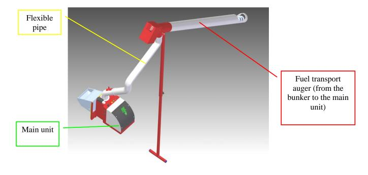
**Figure 3.1** Arrangement of the modules of the pellet burner (top view);
